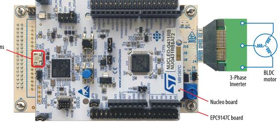
Figure 2: Application overview of the EPC9147C control interface board
