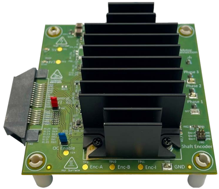
EPC9176 Demonstration board with heatsink attached
