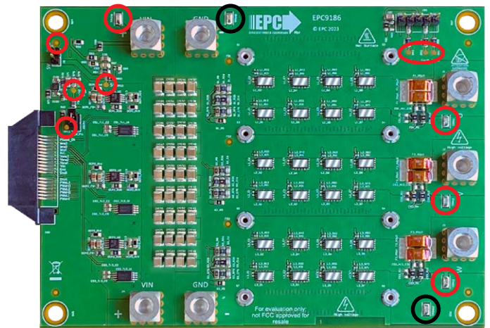
Figure 3: EPC9186 test point pad and hookup locations and designations. In black the PGND reference points.
