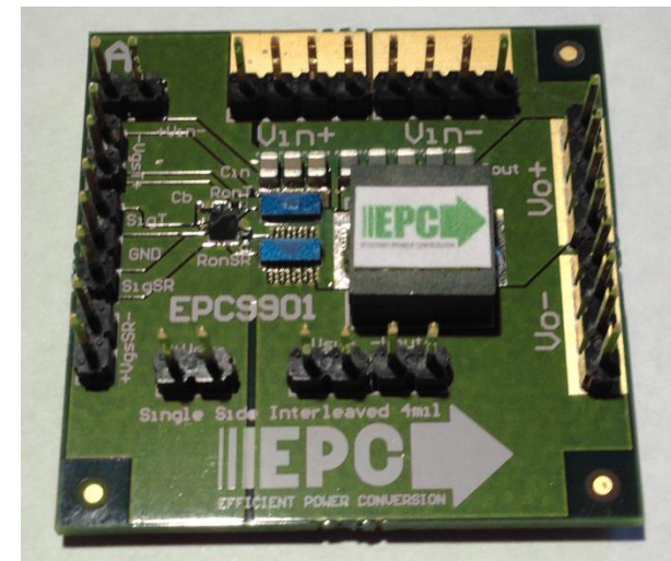
Experimental Prototype L_{LOOP} \approx 0.4 \text{ nH}
