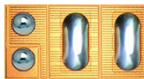
Figure 15: GaN Power Transistor with integrated driver from EPC
