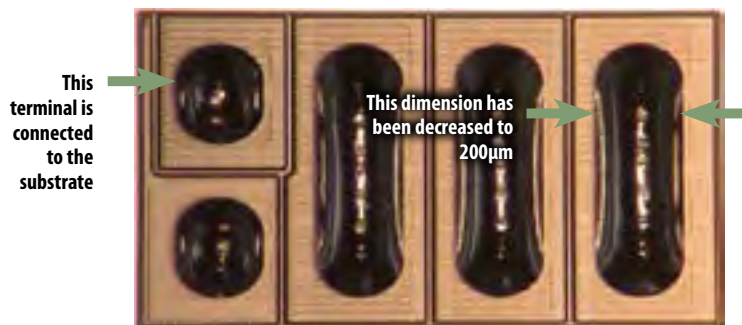
Figure 29: Magnified die photo of EPC2014 and EPC2007 indicating the solder bar that is connected to the silicon substrate and the decreased solder bar width.
